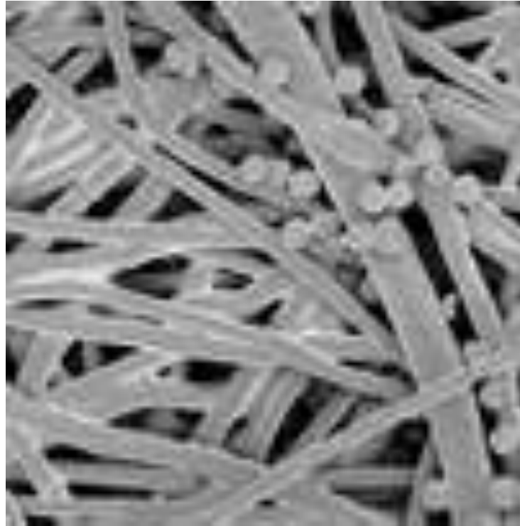
Figure 4. Scanning electronic microscope image showing arrangement of fibres of nonwoven spun-bond fabric layer that creates a torturous filtration path for pollen grains and hence reduce contamination despite larger pore size.
